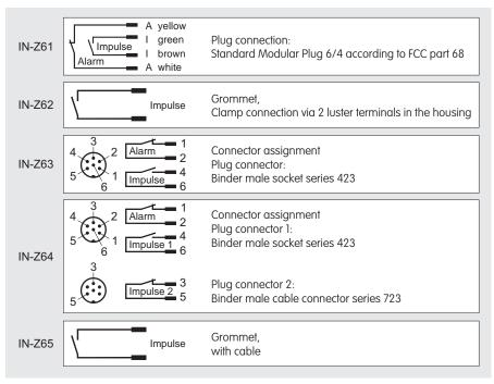
A: Alarm contact, reed switch (normally closed)
