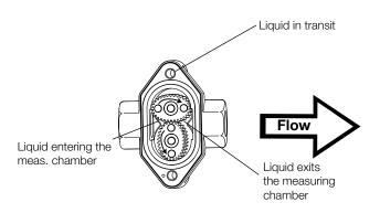
The positive displacement flow technology allows for precise flow measurement of most clean liquids regardless of the media conductivity. Other liquid properties also have a minimal effect on the performance of this type of meter. Flow profile conditioning is not required as with alternative flow technology options making oval gear installations simple to install in tight spaces and at an economical price.
